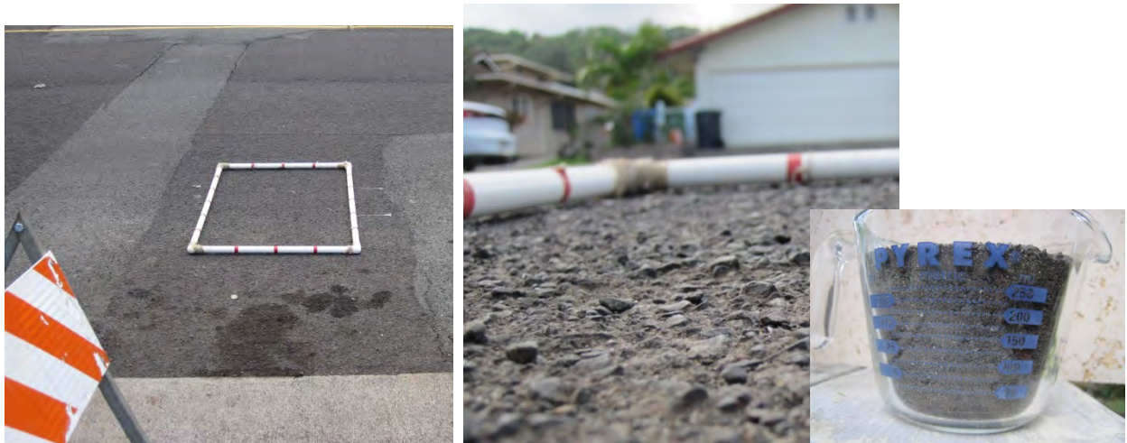
Figure 27 Testing for quantity and quality of material eroded from City road surfaces.
