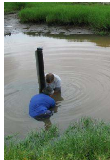
Figure 2. PI and Hugo Defries deploying automated tide sensor, May 30, 2009).
