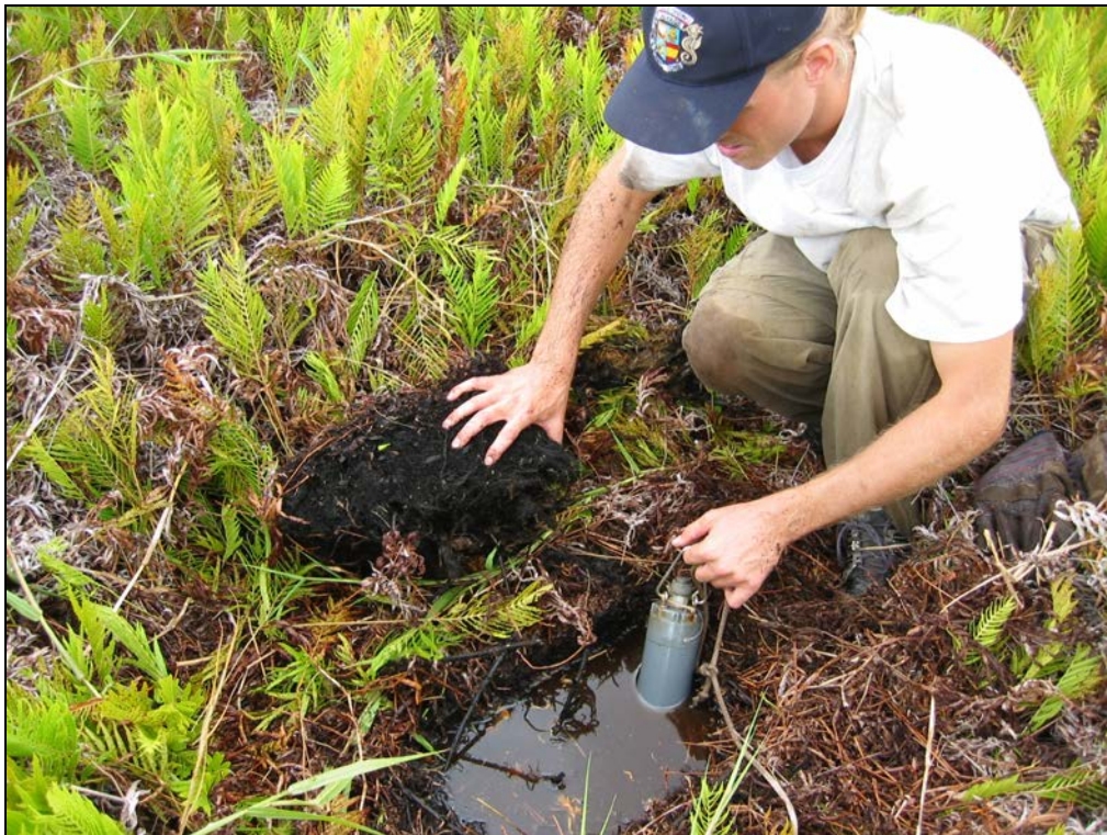
Figure 10. YSI Datasonde deployed in cut-out hole taking water measurements.
