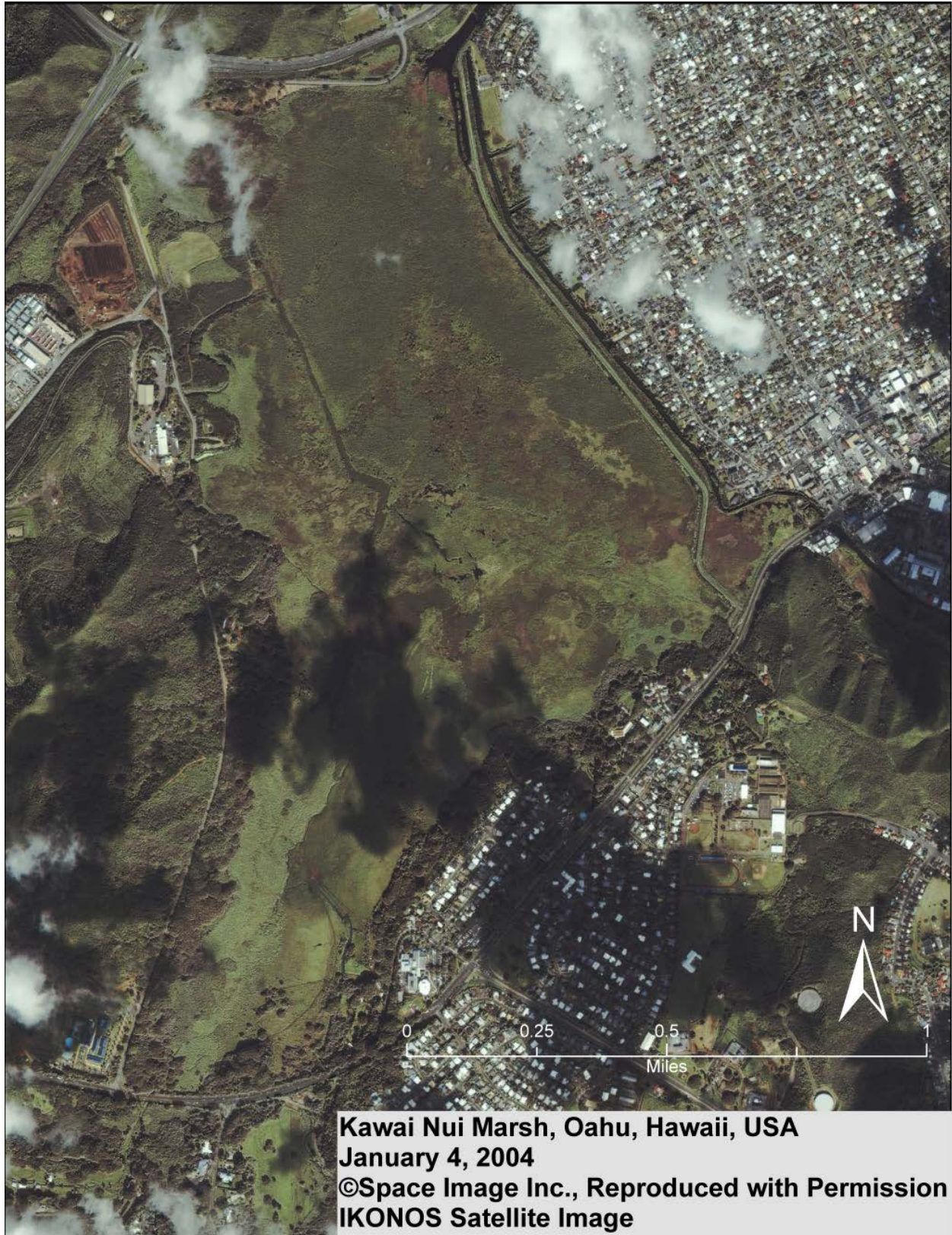
Figure 6. Recent IKONOS Satellite Image of Kawai Nui Marsh (Multi-spectral) used to generate vegetation cover map. Vegetation cover in the cloudy sercacion in the center was discernable using the infrared band.
