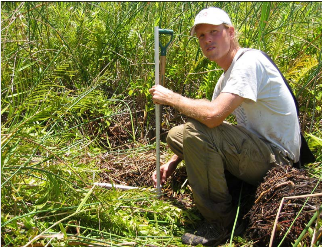
Figure 8. PVC Caliper used to measure peat thickness. The tail of the "L" is under the peat in this photo.
