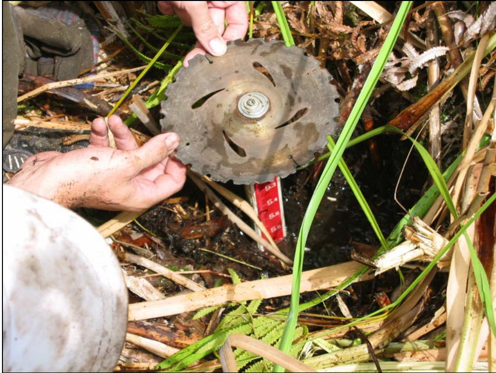
Figure 11. Survey pole with 6-inch metal disc (dulled saw blade) inserted in hole (in this case measuring depth to hard bottom). Depth to mud was measured by reversing the pole and inserting the pole disc first.
