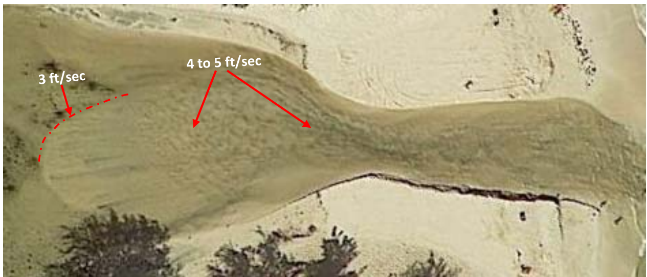
Figure 3.8 Stream mouth opening by storm overflow (1/29/13. Google). Upper photo: Area between Lanikai Bridge and Kailua Beach with ocean current flowing from west to east (top to bottom) and sand being deposited just offshore and to the west (boat ramp) end of Kailua Beach. Lower photo shows how outflowing current erodes sand from the channel as the current speed increases in the narrow channel.
