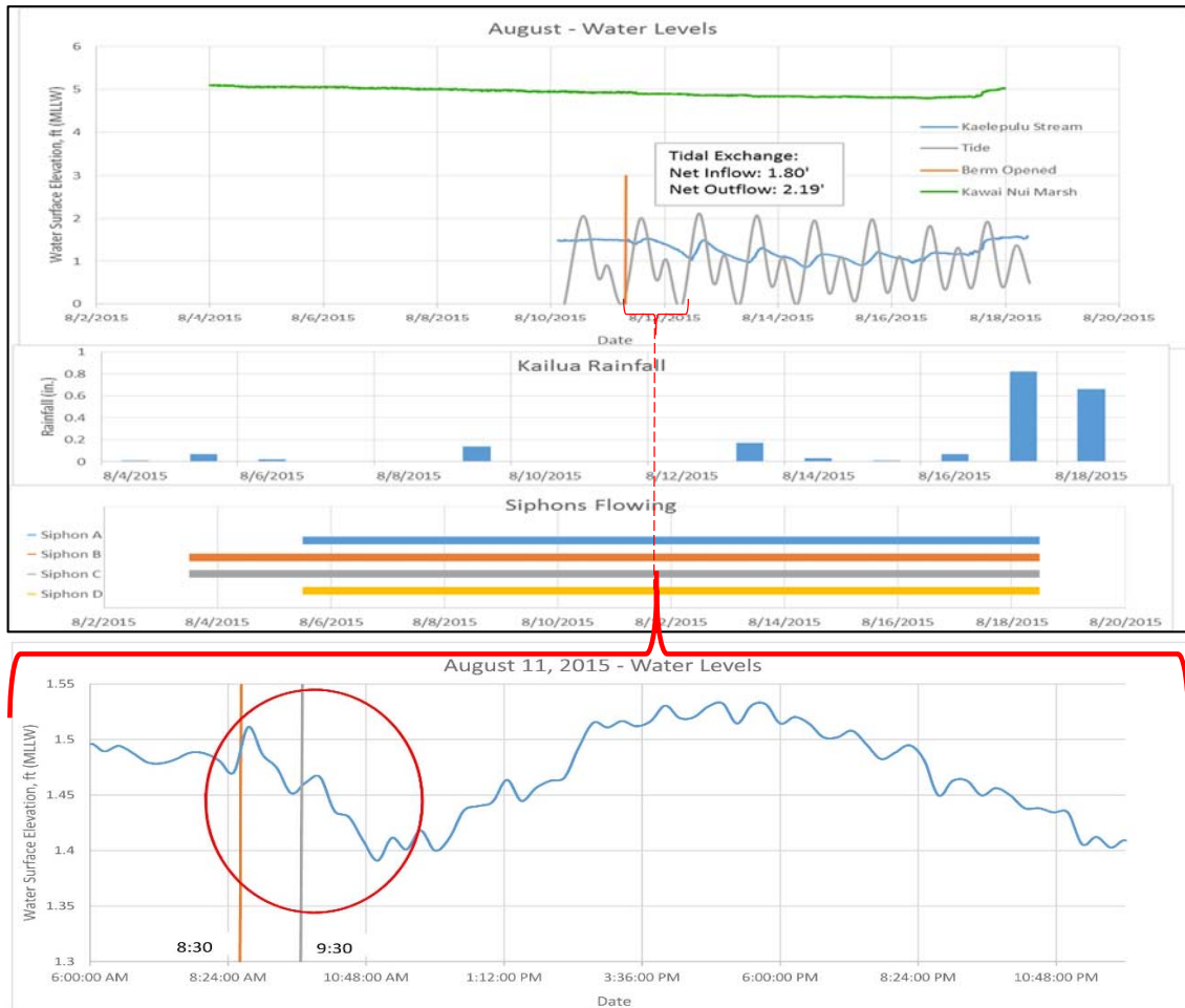
Figure 3.16 August 2015 Water surface elevations and syphon operation.
