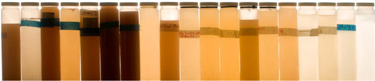
Figure 19 Water quality samples from pond inlets obtained during a single runoff event (3/19/06) distinguish between drainages that have active construction grading projects and those that do not.
