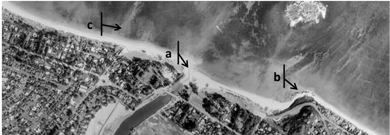
Figure 30 1963 aerial (USGS EKM-2CC-246) dated 1-14-63 prior to construction of Kawainui Levee. Note stream flowing across sand beach (a), and wide sand beach continuous around Aala Point and into Lanikai (b). Location of historic stream mouth channel (~1850 nautical chart) can be seen ~1,000 feet to the west (c).
