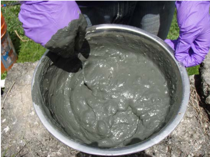
Samples were mixed and composited in stainless steel bowls with a stainless steel spoon
