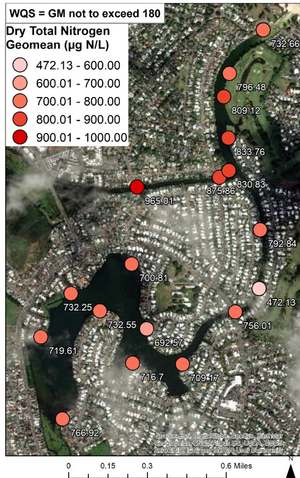
FIGURE 5: GEOMETRIC MEAN OF TOTAL NITROGEN DATA GROUPED BY EVENT TYPE (WET OR DRY EVENT). DATA RANGES REFLECT GM DISTRIBUTION AND THE RELEVANT WATER QUALITY STANDARD. ALL SITES ARE COLORED RED BECAUSE ALL VALUES EXCEED THE GM STREAM STANDARD. THE SHADE OF RED RELATES TO THE MAGNITUDE OF IMPAIRMENT. THE DARKER THE SHADE, THE GREATER THE GEOMETRIC MEAN
