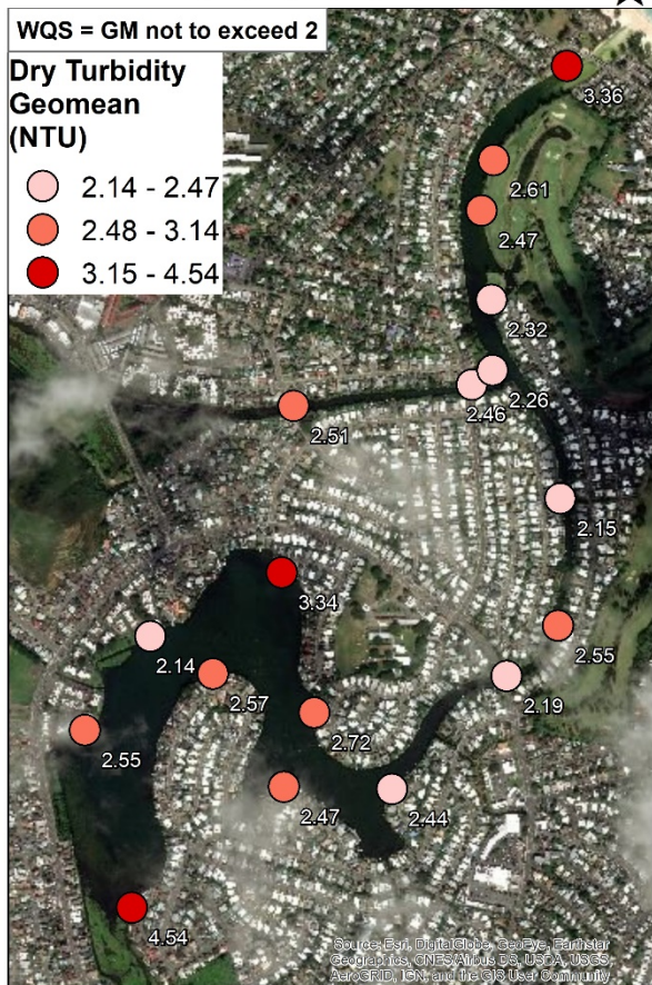
FIGURE 8: GEOMETRIC MEAN OF TURBIDITY DATA GROUPED BY EVENT TYPE (WET OR DRY EVENT). DATA RANGES REFLECT GM DISTRIBUTION AND THE RELEVANT WATER QUALITY STANDARD. SITES THAT MEET THE GEOMETRIC MEAN STREAM STANDARD ARE SHADED GREEN. THE YELLOWER THE SHADE, THE GREATER THE GEOMETRIC MEAN WHILE STILL MEETING THE STANDARD. RED SHADES SYMBOLIZE IMPAIRMENT. THE DARKER THE RED SHADE, THE GREATER THE GEOMETRIC MEAN.
